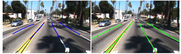
Fig. 10. Post-processing splines. Left: splines before post-processing in blue. Right: splines after post-processing in green. They appear longer and localized on the lanes.
