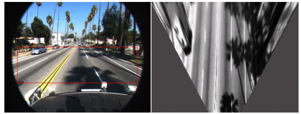
Fig. 3. IPM sample. Left: input image with region of interest in red. Right: the IPM view.
